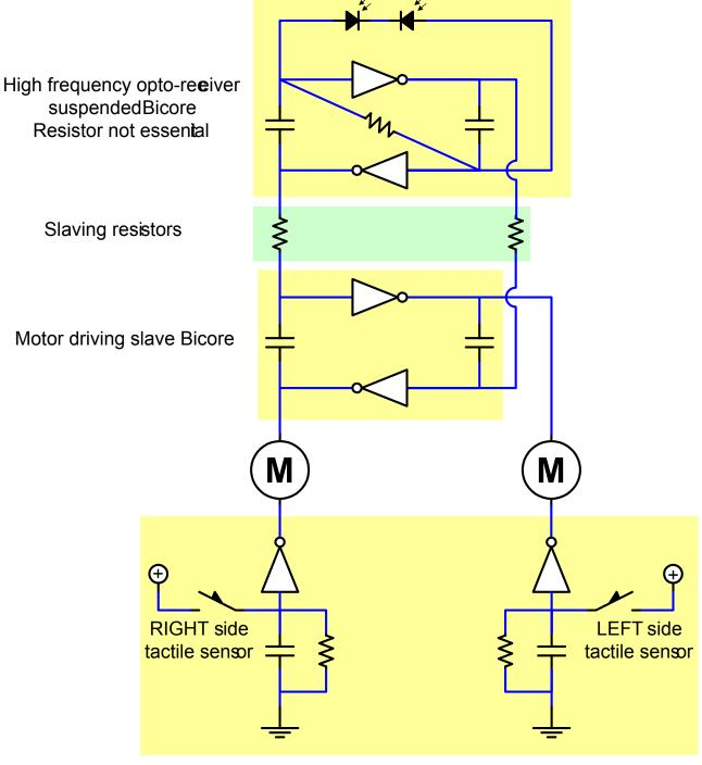
Motor polarity changing circuit (backup with timeut RC circuit)
